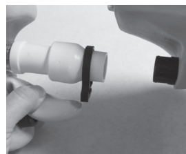
Photo 5 Slide tube to meet ridge on connector:
