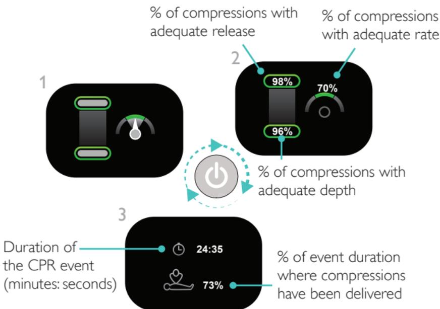
The CPRmeter 2 reverts to Compression Feedback mode if a compression is delivered.
