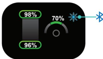
To connect a device, go to the QCPR Quick Review screen by pushing the On/Off button. The status light will flash blue indicating that Bluetooth is on and available for connection. When connected to a device, the flashing blue light turns steady. The CPRmeter 2 is now ready to transfer CPR performance data.
