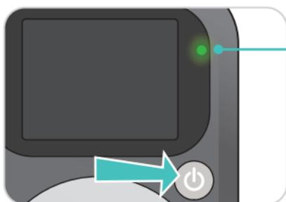
Status Light turns green for a few seconds, when CPRmeter 2 is turned on.
