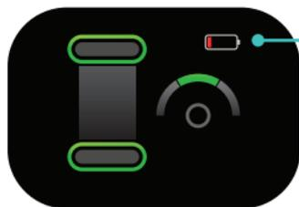
A low-battery icon appears when the CPRmeter 2 is being turned on.
