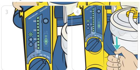
3. The test will start immediately. During test mode, the Power On Indicator will flash rapidly.
