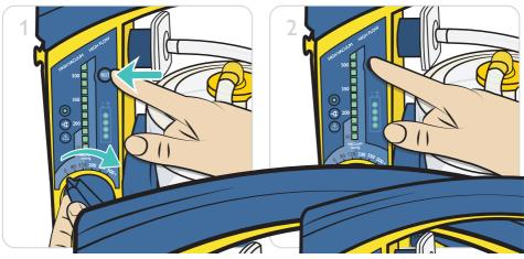
1. Press and hold the Test Button while turning the Operating Knob to 500+ mmHg.
