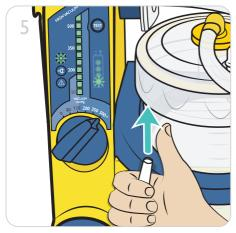
5. Keep the tubing blocked while LED 2, 3 and 4 light up. Release the tubing when LED 1 lights up again.
