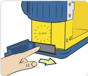
4. To insert a battery, push it fully in and then to the right to lock it.
