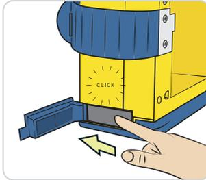
2. To remove the battery, push and move it slightly to the left and then release.
