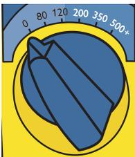
The LSU is switched ON by turning the Operating Knob to the required setting. Each setting indicates the maximum achievable vacuum level for the selected position (80, 120, 200, 350, 500+ mmHg). The free air flow value changes along with the increasing vacuum settings (see section 9.4 for details). The LSU is switched OFF by resetting the Operating Knob to "0".
