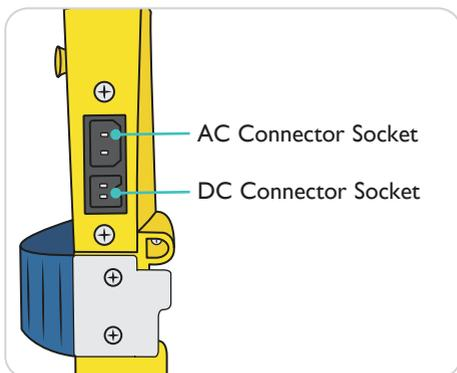
External power connection will cause the External Power Indicator to be lit.
