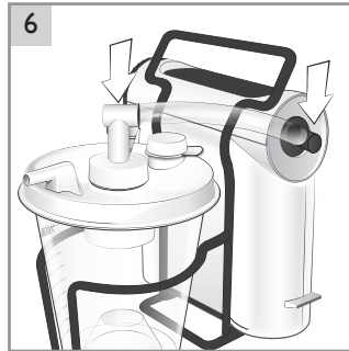
6 Check that all Vacuum Tube connections are firmly attached.
