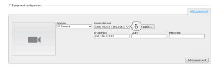
Figure 21 IP camera search finished and drop-down list ready
