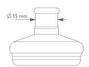
Pressure release valve: Upright has a pressure release valve ("pop-off") which limits the airway pressure to 30-45 cmH<sub>2</sub>O. A hissing sound can be heard when the valve opens. If higher airway pressure is needed, press downwards on the valve with the index finger while squeezing the bag.
