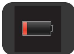
**IMPORTANT NOTE:** *If the remaining battery power during use becomes too low to sustain further operation, the battery-low icon is shown for 10 seconds and then the CPRmeter turns itself off.*
