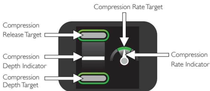
The display of the CPRmeter provides real-time feedback to the responder as described below.
