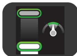
If the CPR meter detects a compression that exceeds 70 mm (2.75"), the CPRmeter shows the depth indicator below the target area. If a specific CPR event requires CPR to be performed on a patient lying on a mattress, slide a backboard under the patient and compensate for the mattress softness by ensuring that for each chest compression the area below the compression depth target lights up.
