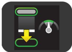
If 4 consecutive compressions fail to meet the compression depth target, the display shows a yellow arrow pointing to the compression depth target.
