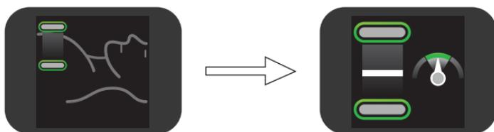
3. Follow feedback provided by the indicators on the CPRmeter display. The indicators are described in the following section. If no CPRmeter feedback is observed, remove the CPRmeter and begin chest compressions.
