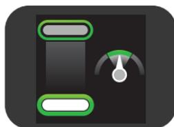
If the CPRmeter detects that the rate of compressions is within the target area, the "speedometer" needle on the compression rate indicator points to the green target area and the green target briefly illuminates.
