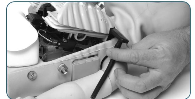
Remove bladder from site cavity by sliding it sideways out of the chest.
