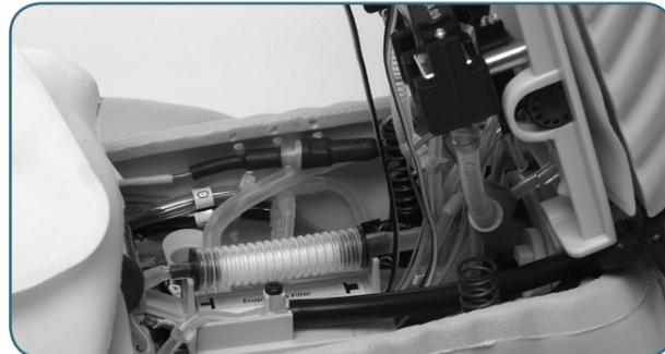
Lift the chest plate assy exposing the internal parts and find the filter holder.
