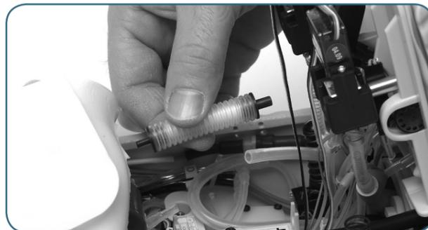
Disconnect the filter assy and replace with a new one.
