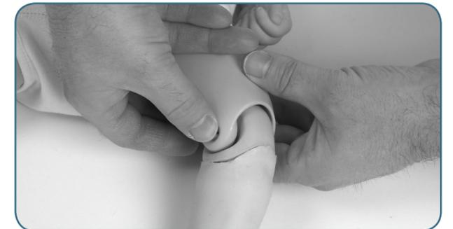
Press the bolt in the knee part out of its seat.
