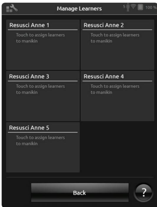
To manage a large group of learners, you can import a list of names to SimPad. Connect SimPad to a computer; using the SimPad-to-PC cable that comes with SimPad. SimPad appears as an external disk drive on your computer.
