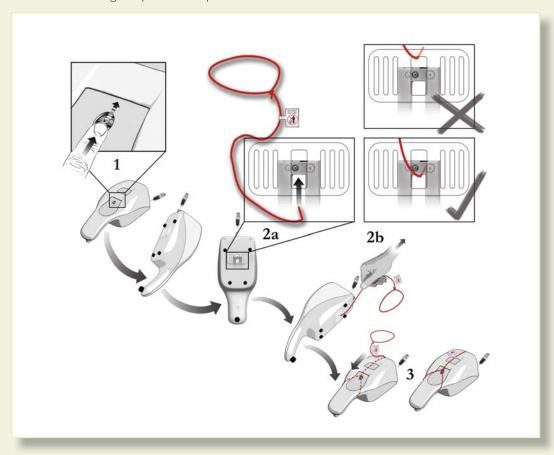
(5) Carefully place the haptic device and tools in the original packaging:
