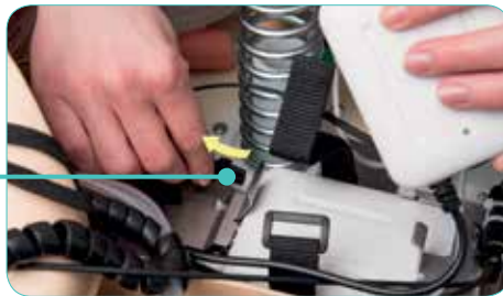
Detach battery connector from Link Box.
