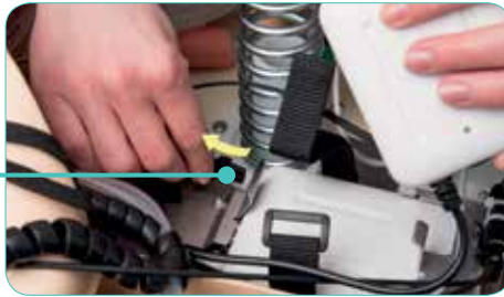
Detach battery connector from Link Box.
