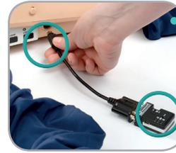
For SkillReporter manikins, connect the Bluetooth manikin adapter to the manikin using the supplied cable. A red light indicate that the adapter is ready for use.
