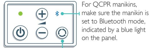
For QCPR manikins, make sure the manikin is set to Bluetooth mode, indicated by a blue light on the panel.
